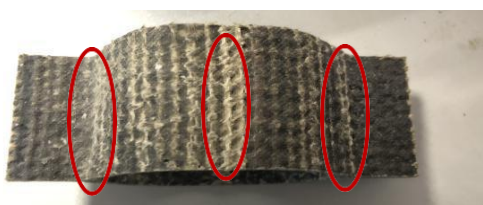
(a) Failure modes of special-shaped 3D circular tubular woven composites
