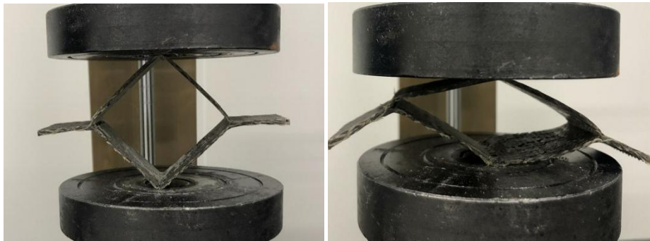
(c) Special-shaped 3D square tube composite material compression process of 1mm
