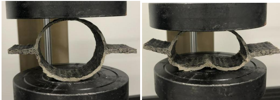
(b) Special-shaped 3D circular tube composite material compression process of 2 mm
