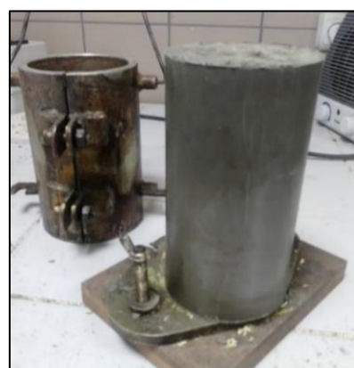
Figure 7. Cylinder SPC sample after one hour
