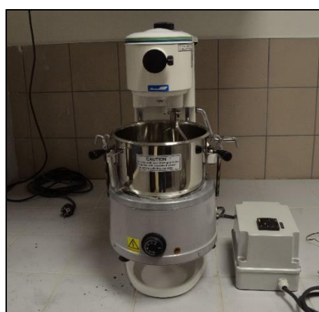
Figure 1. Temperature-controlled mechanical mixer
