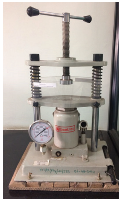
Figure 1. Camera image of the KBr press used to form tablets.
