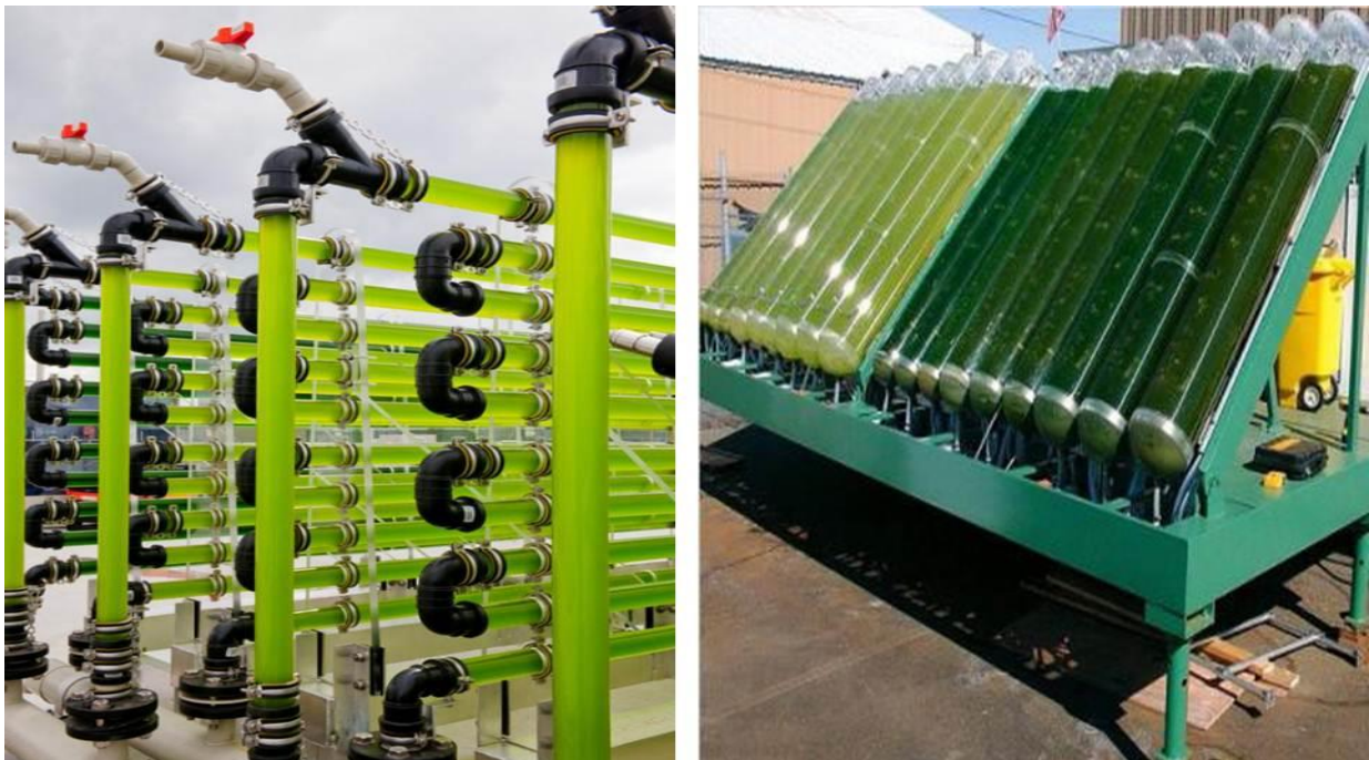
Figure 1. Closed cultivating system units for algal biomass production
