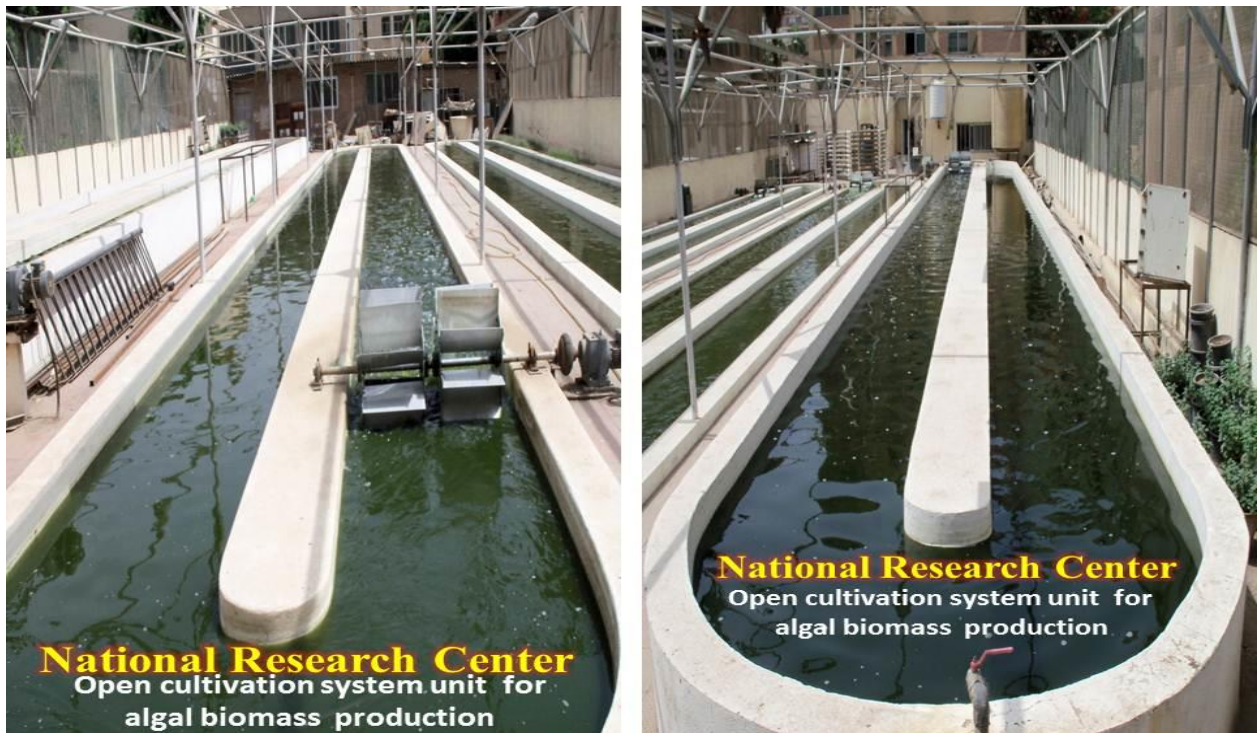
Figure 2. Open cultivation system unit for algal biomass production
