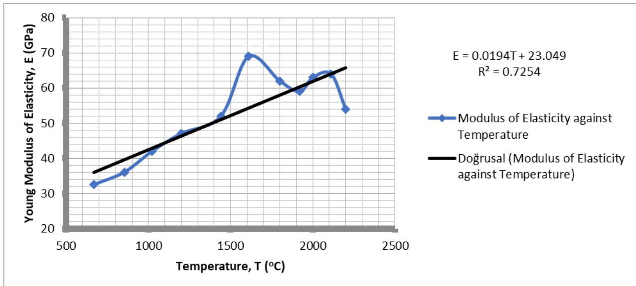
**Fig. 4.** Graph of the Effect of Temperature on the Modulus of Elasticity of the Developed Aluminium Sheet
