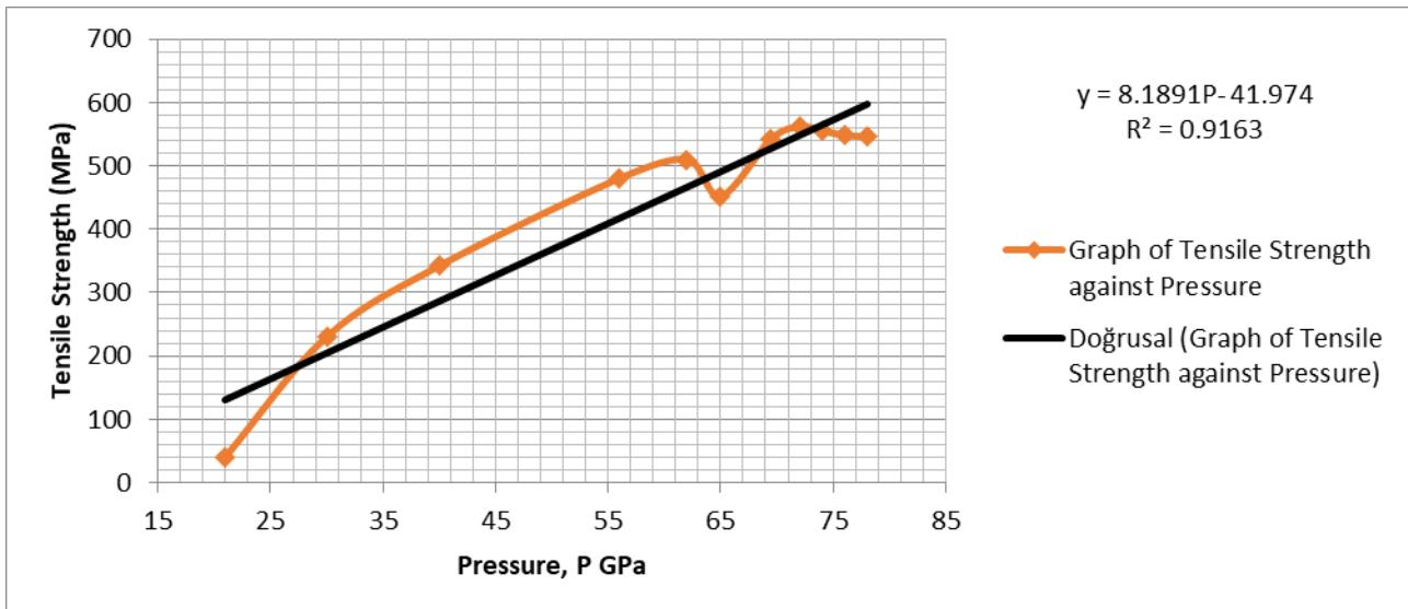
Fig. 3. Graph of the Effect of Pressure on the Tensile Strength of the Developed Aluminium Sheet
