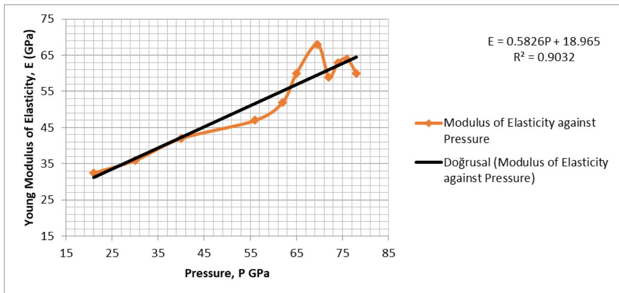
**Fig. 5.** Graph of the Effect of Pressure on the Modulus of Elasticity of the Developed Aluminium Sheet
