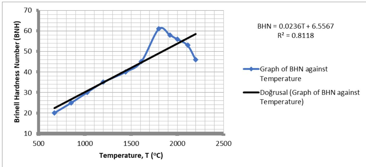
Fig. 8. Graph of the Effect of Temperature on the Brinell Hardness Number of the Developed Aluminium Sheet
