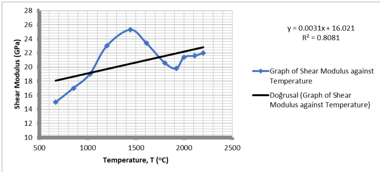
**Fig. 6.** Graph of the Effect of Temperature on the Shear Modulus of the Developed Aluminium Sheet
