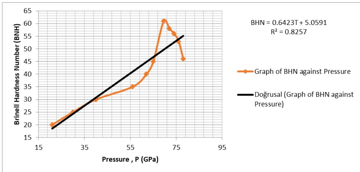
Fig. 9. Graph of the Effect of Pressure on the Brinell Hardness Number of the Developed Aluminium Sheet
