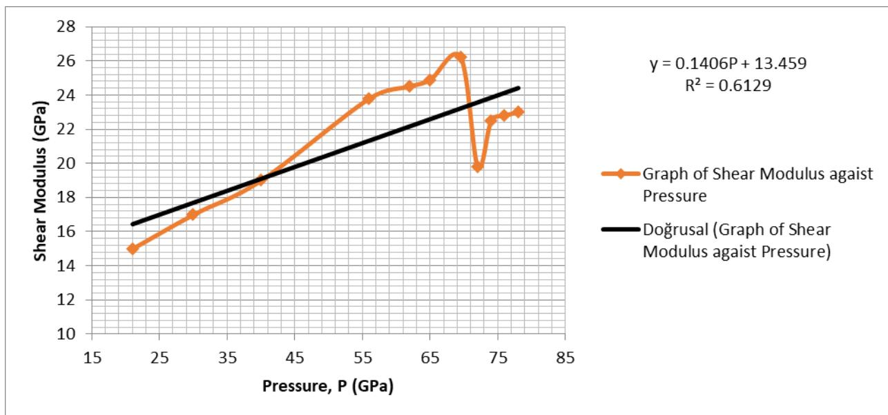
**Fig. 7.** Graph of the Effect of Pressure on the Shear Modulus of the Developed Aluminium Sheet
