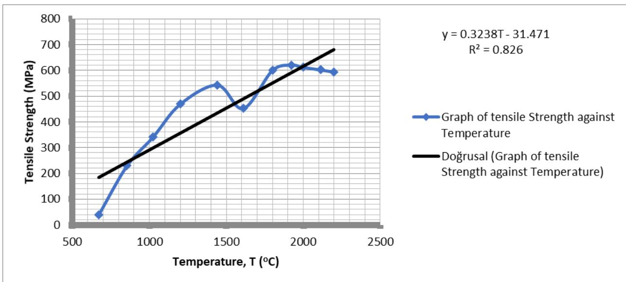
Fig. 2. Graph of the Effect of Temperature on the Tensile Strength of the Developed Aluminium Sheet
