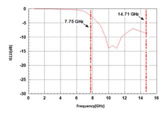
**Figure 3.** Return loss values (S11 parameter) of dipole antenna versus frequency
