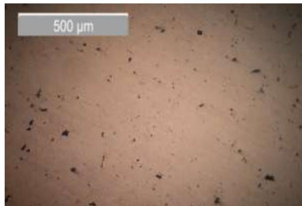
**Figure 3.** Microstructural images of the aluminum sample manufactured using P/M prior to sintering process
