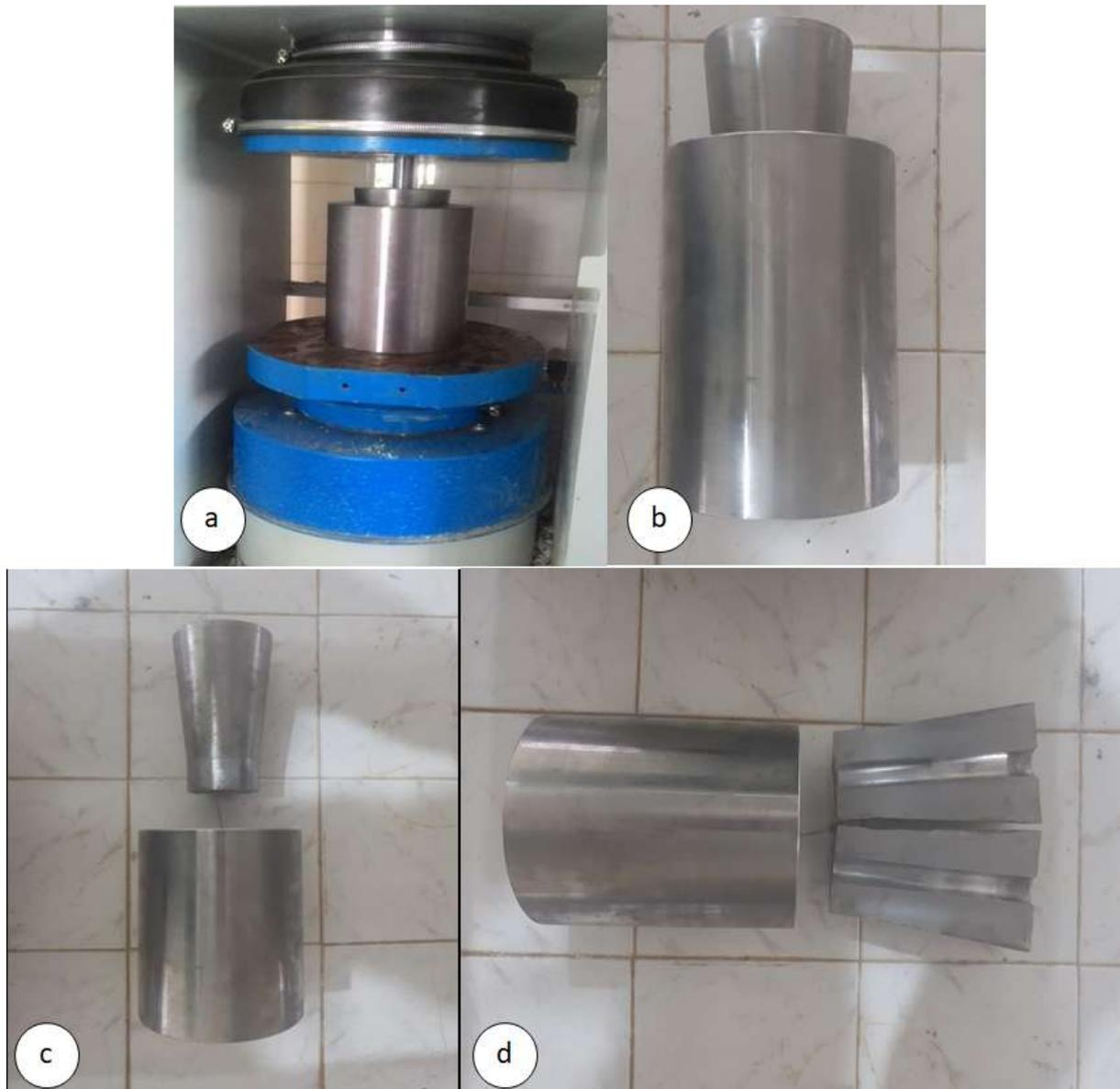
**Figure 1.** a) Pressing, b-d) Removal of samples following the pressing process
