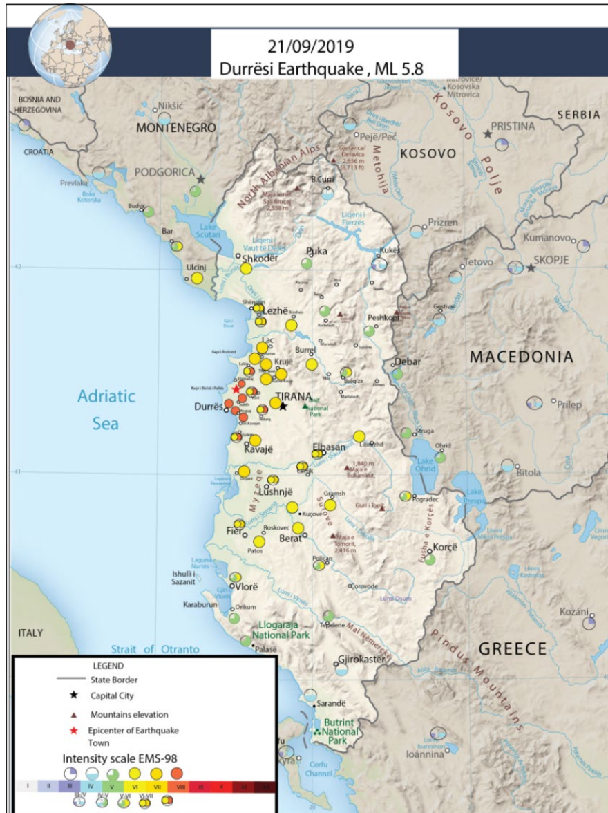
Figure 3. Municipality macroseismic EMS-98 intensities assessed using 1175 questionnaires, compiled through the seismicity site ( www.geo.edu , www.emsc-csem.org ), and questionnaires compiled by EMSC and other alternative way. The purple star represents the instrumental epicenter. The inset shows an enlargement of the epicentral area (Ormeni et al 2019). The attenuation of Intensity versus the epicentral distance was then fitted with a 2nd degree polynomial function for Durrësi earthquakes respectively [Eq. 2]:
