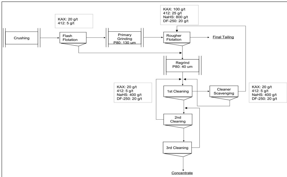
Figure 4. Flowsheet of the locked cycle flotation test
