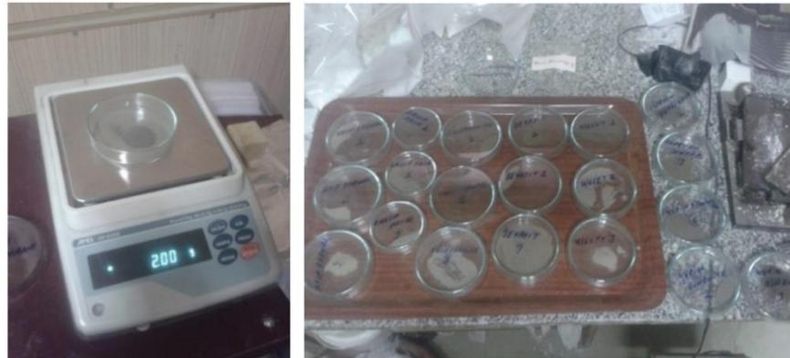
**Fig. 1.** Weighed soil samples (left) and all samples in the petri dishes after sieving (right).
