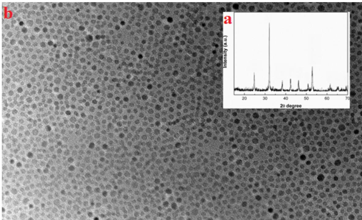
**Figure 1.** a-X ray diffraction pattern and b-Transmission electron microscope (TEM) image of iron oxide NPs.
