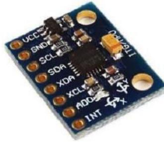
Figure 1. MPU6050 IMU sensor card
