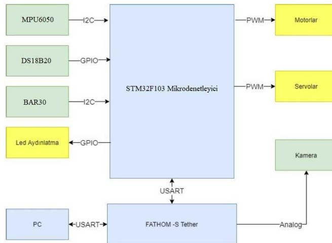
Figure 5. Block diagram of the designed system
