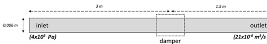
Figure 3. Geometric configuration of the solution domain.
