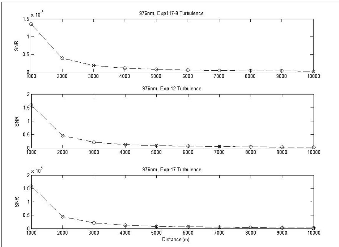
Figure 8. 976 nm wavelength turbulence conditions and SNR.
