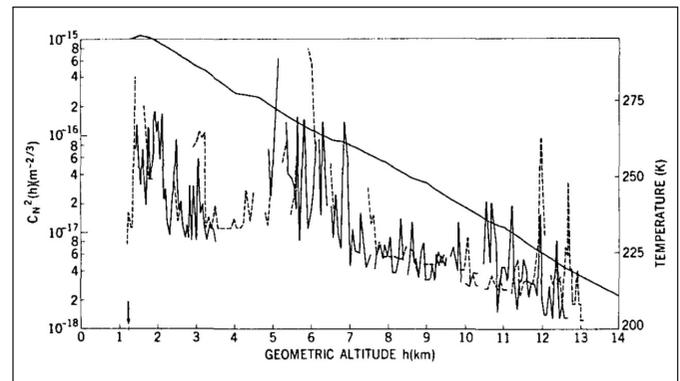
**Figure 1.** Refractive-index-structure coefficient and temperature vs altitude. (Diagonal line is the corresponding temperature profile. Arrow indicates altitude of launch site.)
