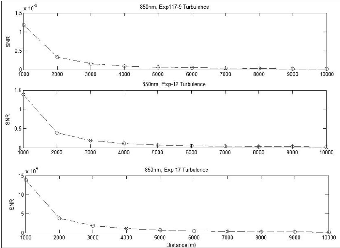
Figure 7. 850 nm wavelength turbulence conditions and SNR.
