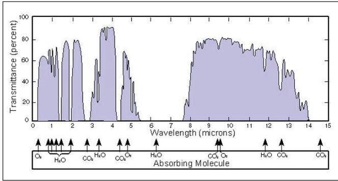
**Figure 4.** Clear air atmospheric transmission windows.
