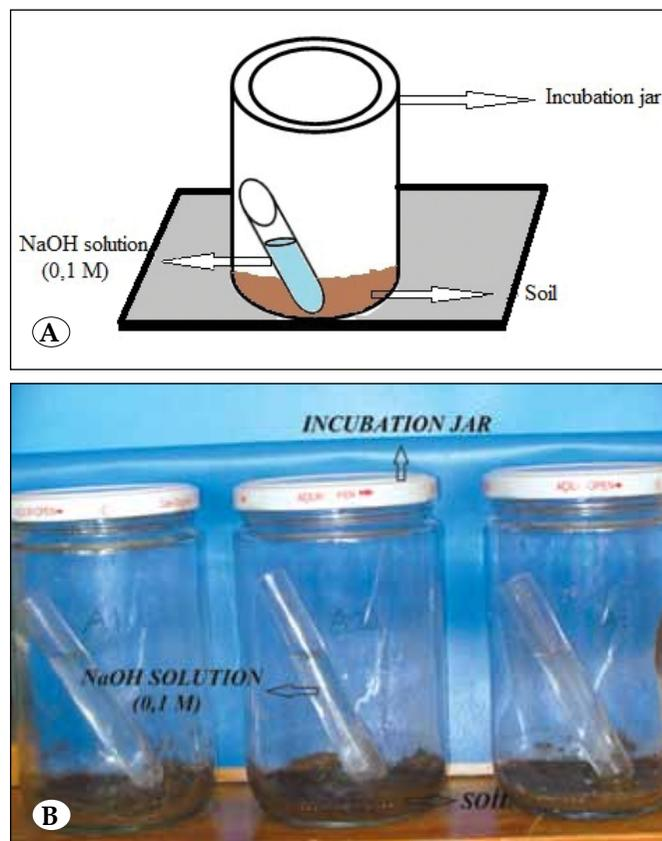
**Figure 1:** A) The experimental setup used to measure the CO<sub>2</sub>-C evolution rates. B) Three replicates of one of the reactor.
