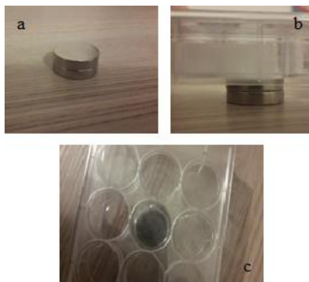
Fig. 1. Two cylindrical Neodymium-Iron-Boron (Nd 2 Fe 14 B) magnets provided the 328 mT SMF. a) All magnets were placed top on top, b) Assay wells of 12-well plates were put on surface of the magnets, c) Each of the magnets had enough surface area to cover interior surface of a well.
