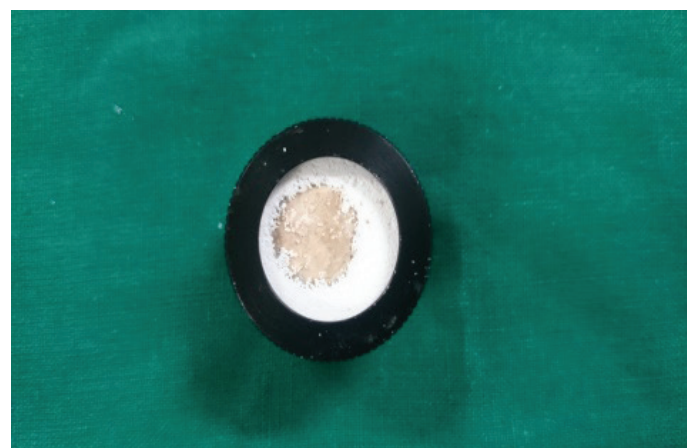
Figure 3. Specimen preparation before placing in the spectrophotometer.
