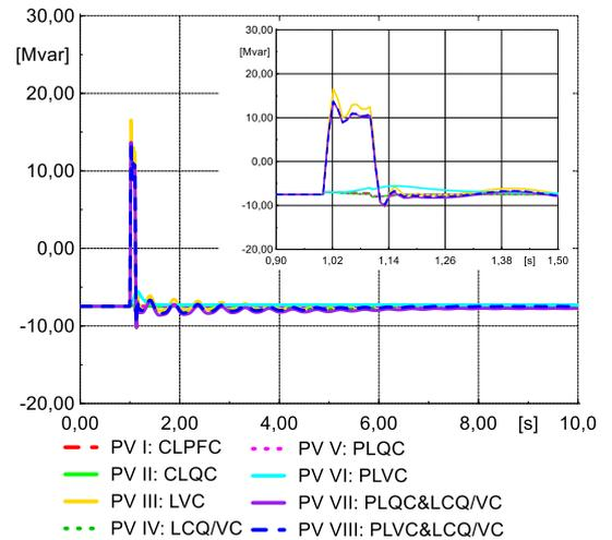
Figure 11 Reactive power of the PV plant with the deactivation of Line 6-9
