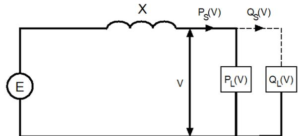
Figure 1 Equivalent circuit of the separated presentation of active and reactive power [22]
