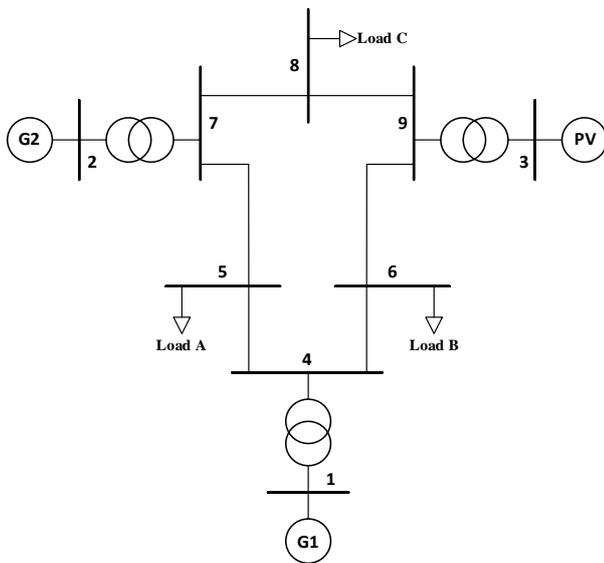
Figure 2 The modified IEEE 9-bus power system
