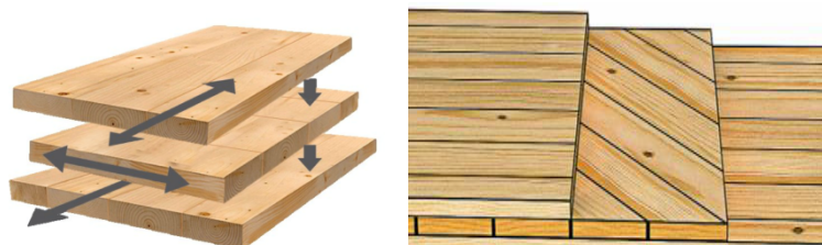
Figure 1: Draft of cross laminated timber
