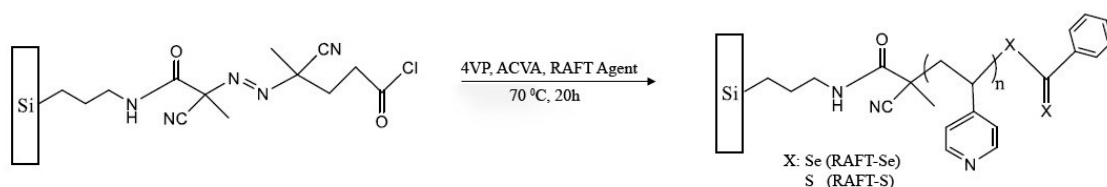
Scheme 4. Schematic diagram illustrating the process of the surface-initiated RAFT polymerization of 4VP from the Si-Azo surface [50].
