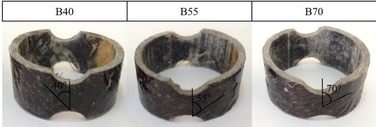
**Figure 3.** The BFRP ring-shaped samples for split disk experiments
