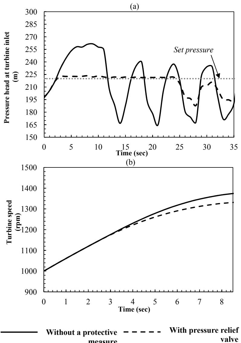
Figure 4. (a) Turbines' inlet pressure; (b) Turbines' speed rise for Scenario B
