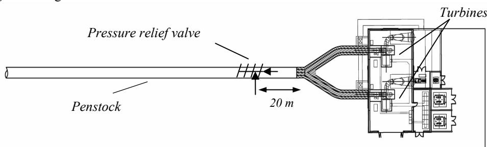
Figure 3. Plan view of the pressure relief valve and powerhouse
