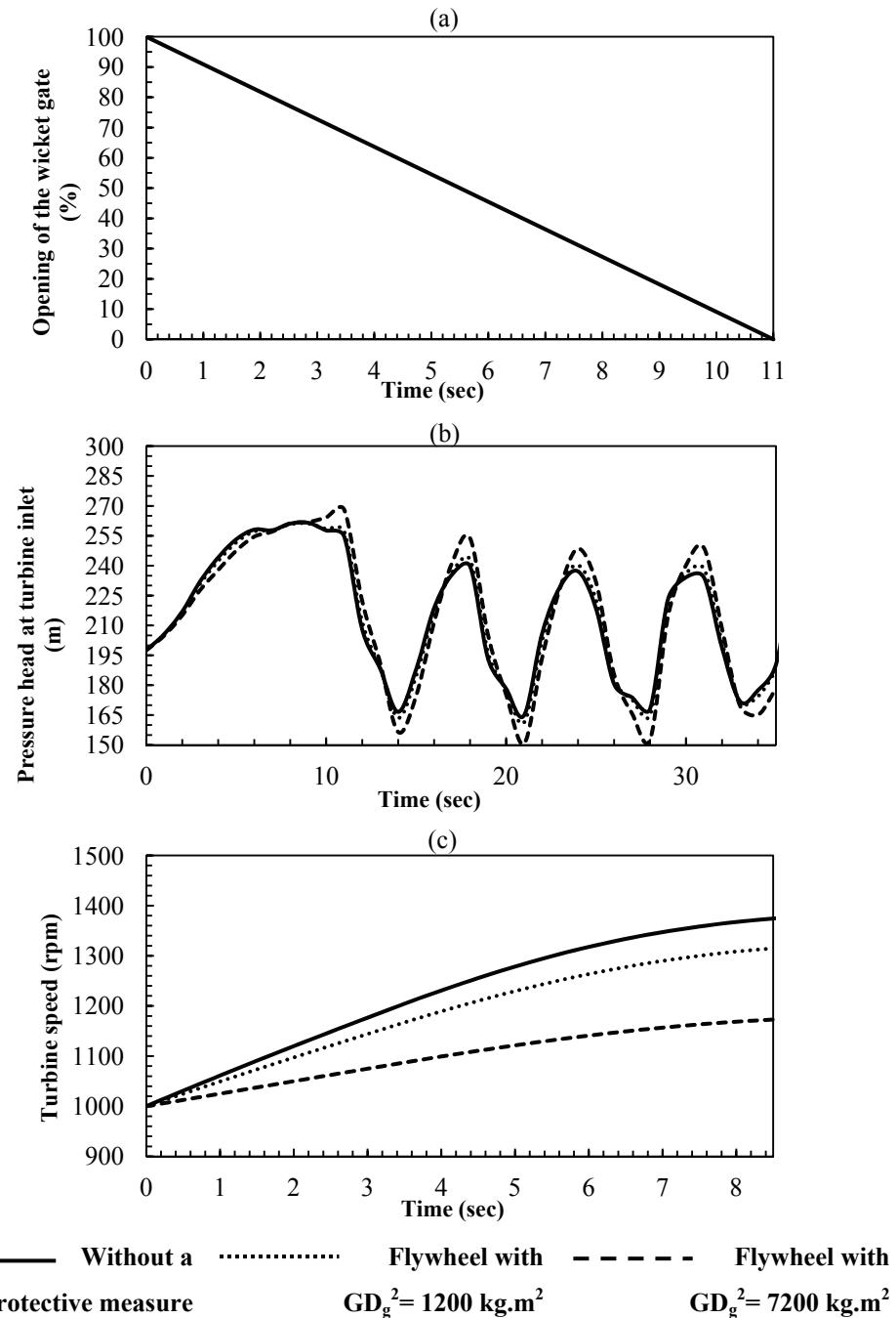
Figure 2. (a) Closure law, (b) Turbines' inlet pressure, (c) Turbines' speed rise
