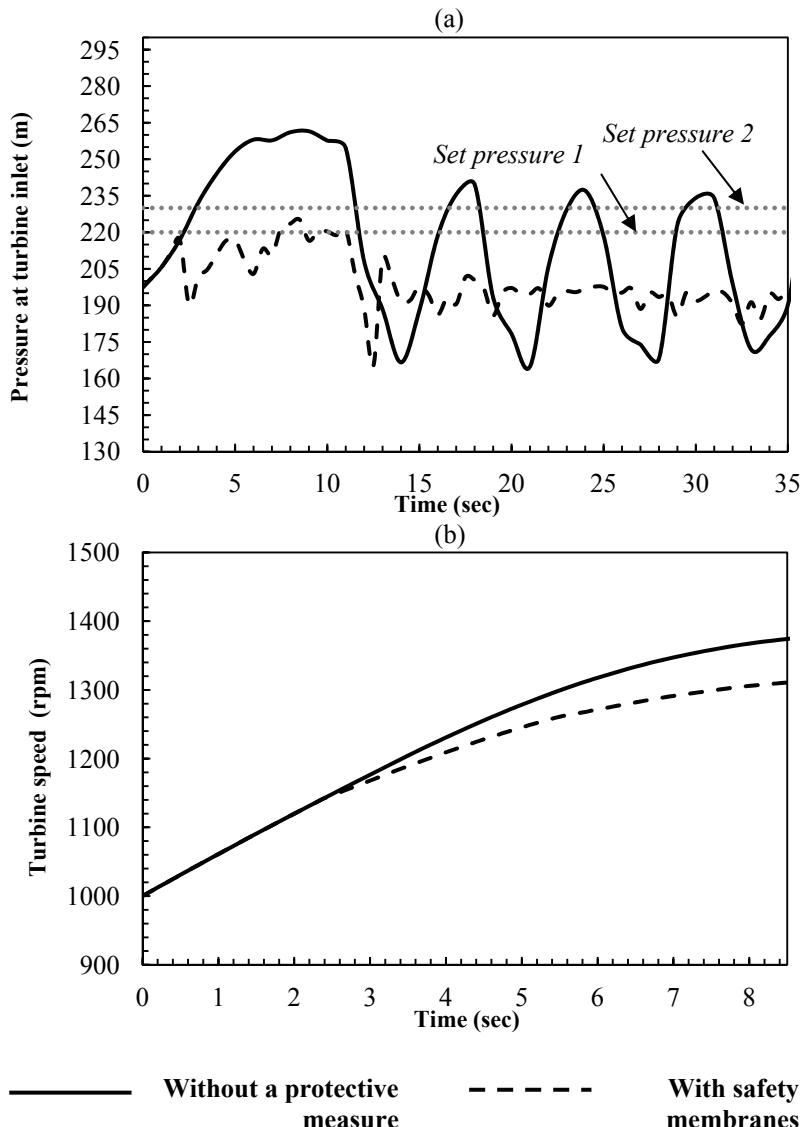
Figure 6. (a) Turbines' inlet pressure; (b) Turbines' speed rise for Scenario C
