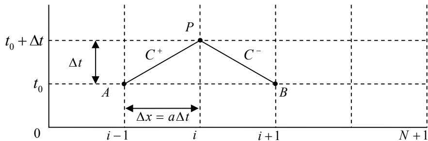
Figure 1. Characteristic lines in time-space domain
