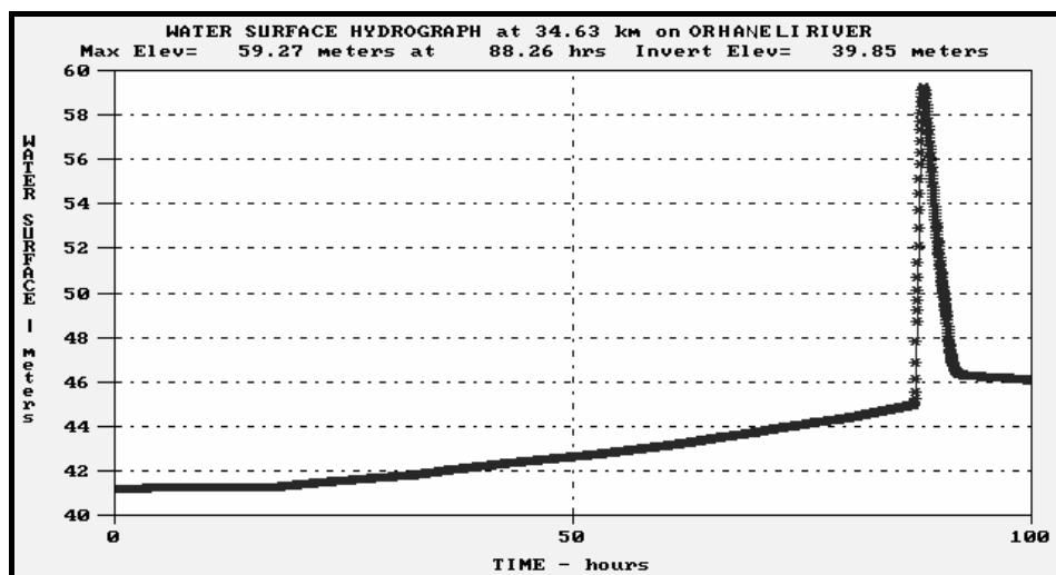
Figure 6. Water Surface Hydrograph at Cross-Section (km: 34.63)
