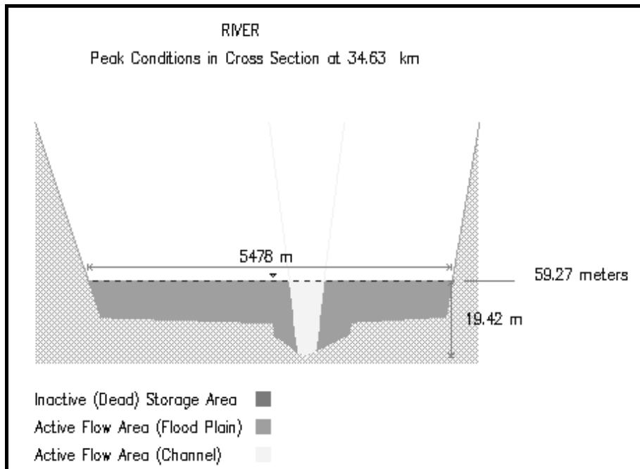
Figure 5. Maximum Water Surface Elevation at Cross-Section (km: 34.63)
