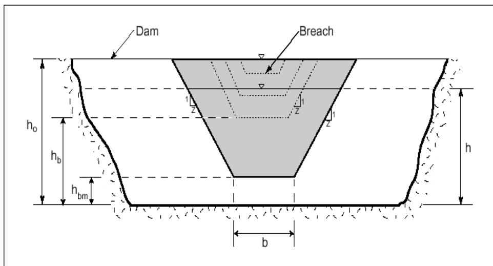
*Figure 3. Geometrical Definition of Breach Parameters*
