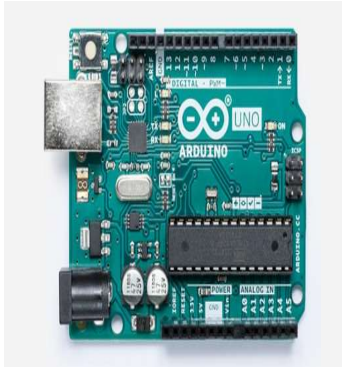
Figure 1. Arduino uno ( https://store.arduino.cc , 2019)
