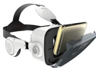
Figure 7. Mounting phone to virtual reality headset
