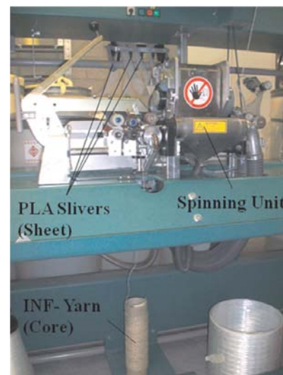
Figure 7. Composite yarn manufacturing by using DREF Spinning Technology.
