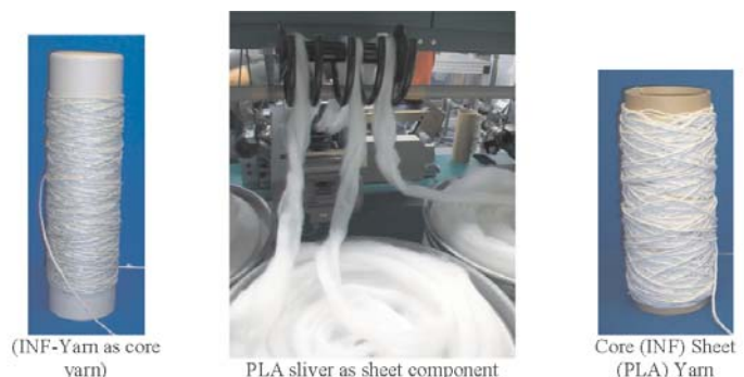
Figure 8. Yarn manufacturing by using DREF Spinning Technology.
