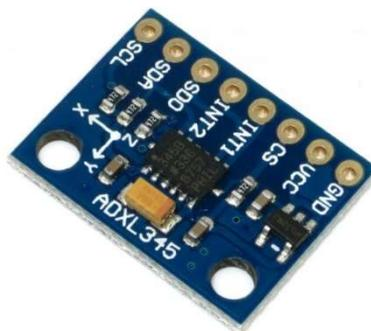
**Figure 3.** ADXL 345 triaxial accelerometer
