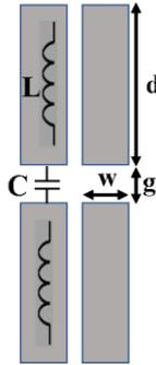
Figure 3. Sample FSS and its EC parameters.
