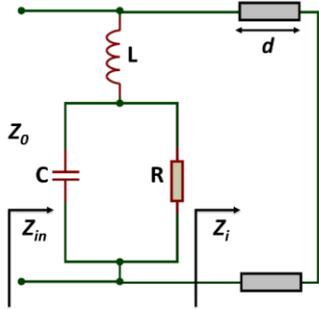
Figure 2. Equivalent circuit model of the FSAS.
