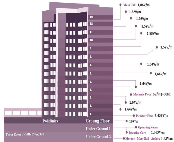
Figure 9. The highest electric field intensity values at 100kHz-8GHz frequency and power frequency measured on each floor.
