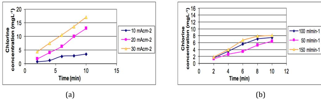
**Figure 4.** Effect of Iridium metal-oxide electrodes on the amount of chlorine production according to (a) current density in parallel plate reactor with flow rate 150 ml/min; (b) flow rate in parallel plate reactor, current density 30 mA/cm<sup>2</sup>.
