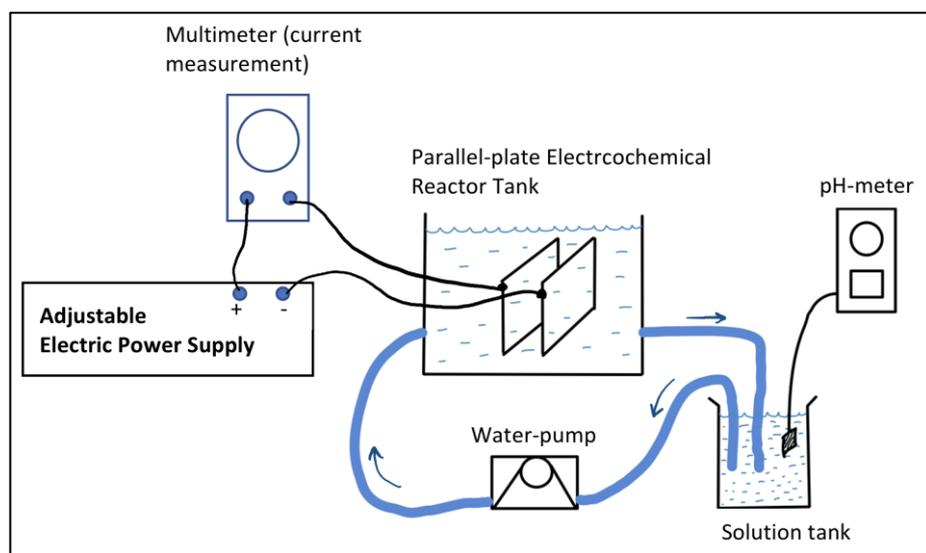
**Figure 1.** Electrochemical reactor setup.
