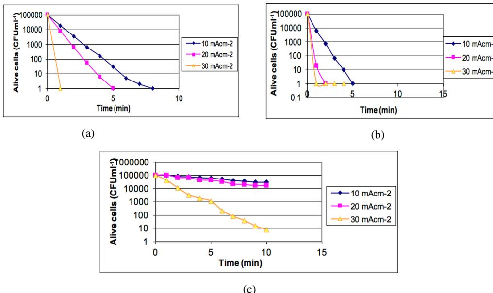
**Figure 2.** Effect of current density on cell survival rate with (a) Boron-doped diamond electrodes, (b) Iridium metal-oxide electrodes, (c) graphite plate electrodes, all in parallel plate reactor.
