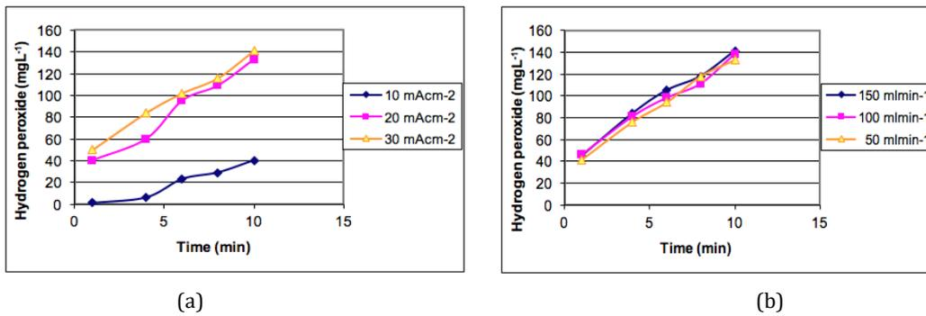
**Figure 7.** Using Iridium metal-oxide electrodes in parallel plate reactor; effect of (a) current density at flow rate of 150 ml/min, (b) flow rate at current density of 30 mA/cm<sup>2</sup>.
