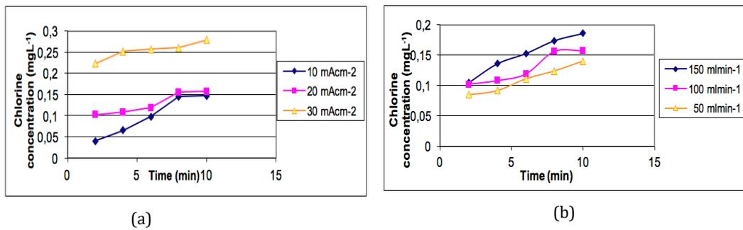
**Figure 5.** Effect of Graphite plate electrodes on the amount of chlorine production according to (a) current density in parallel plate reactor with flow rate 150 ml/min; (b) flow rate in parallel plate reactor, current density 30 mA/cm<sup>2</sup>.
