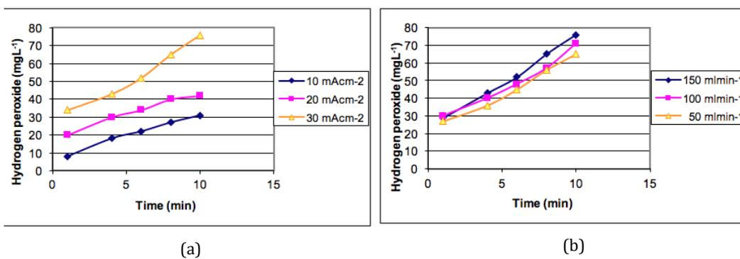
**Figure 8.** Using Graphite plate electrodes in parallel plate reactor; effect of (a) current density at flow rate of 150 ml/min, (b) flow rate at current density of 30 mA/cm<sup>2</sup>.
