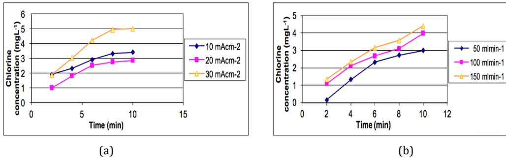
**Figure 3.** Effect of Boron-doped diamond electrodes on the amount of chlorine production according to (a) current density in parallel plate reactor with flow rate 150 ml/min; (b) flow rate in parallel plate reactor, current density 30 mA/cm<sup>2</sup>.
