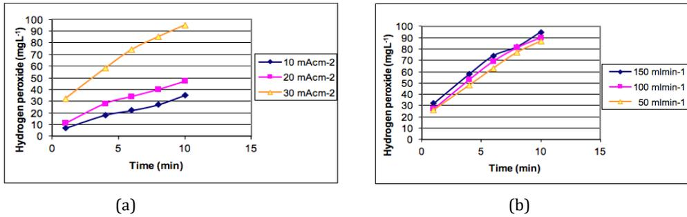
**Figure 6.** Using Boron-doped diamond electrodes in parallel plate reactor; effect of (a) current density at flow rate of 150 ml/min, (b) flow rate at current density of 30 mA/cm<sup>2</sup>.
