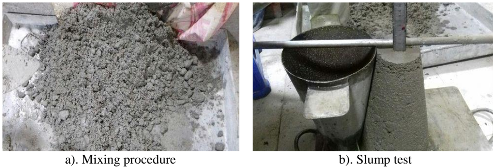
Figure 2. Preparation of concrete and test of workability
