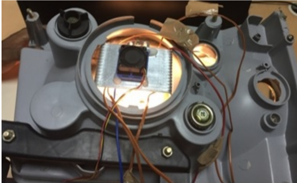
Figure 4. Headlamp assembly with heatsink and cooling fan
