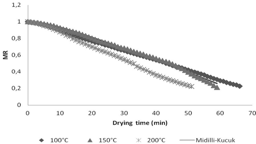
**Figure 2.** Variation of experimental and predicted moisture ratio by Midilli-Kucuk model with drying time at selected temperatures.
