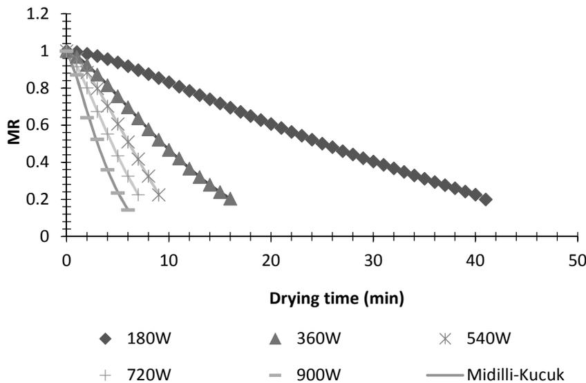
**Figure 1.** Variation of experimental and predicted moisture ratio by Midilli-Kucuk model with drying time at selected microwave output powers
