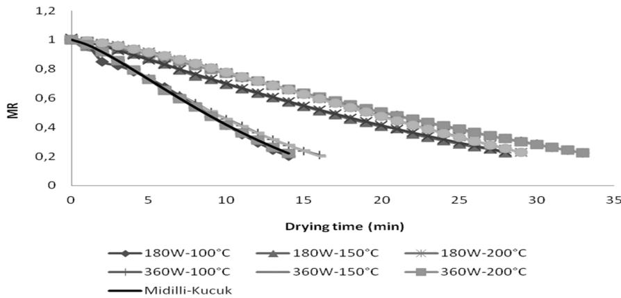
**Figure 3.** Variation of experimental and predicted moisture ratio by Midilli-Kucuk model with drying time at selected temperatures and 180W and 360 W microwave powers.
