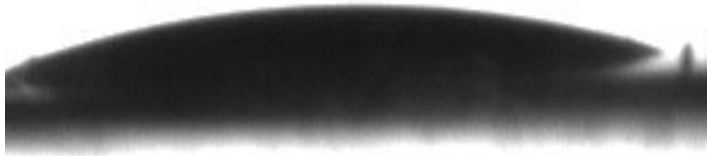
Figure 3.2. Contact Angle Image of TiO_2 Coated Glass
