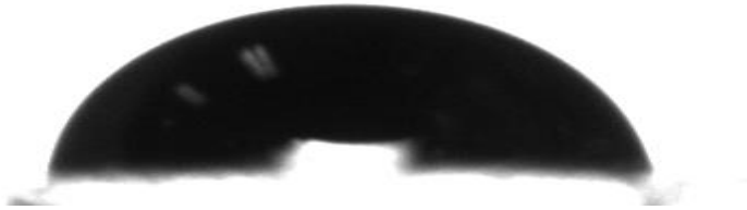
Figure 3.1. Contact Angle Image of Uncoated Glass
