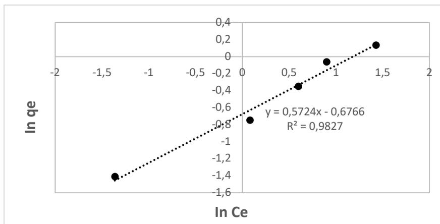
**Figure 6.** Linear graph of Freundlich isotherm for MG biosorption dye onto sunflower straw
