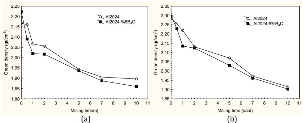
Fig. 3 The change of green density of Al2024 alloy and Al2024-5%B<sub>4</sub>C composite, (a) 300 MPa, (b) 400 MPa
