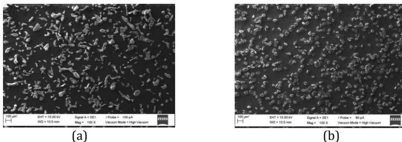
**Fig. 1** Morphology of as-received powders: (a) Al2024 powders and (b) B<sub>4</sub>C particles
