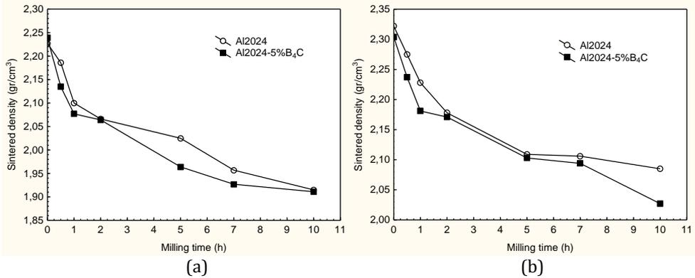
**Fig. 4** The change of sintered density of Al2024 alloy and Al2024-5%B<sub>4</sub>C composite, (a) 300 MPa, (b) 400 MPa
