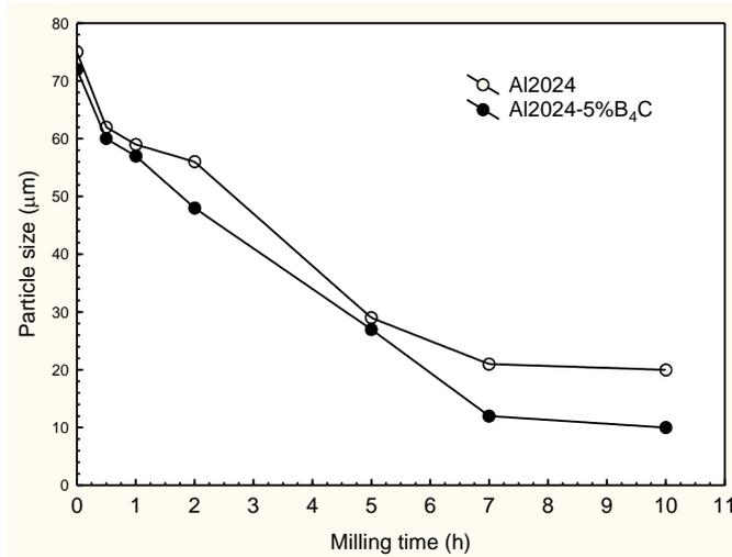
Fig. 2 The change of particle size with increasing milling time
