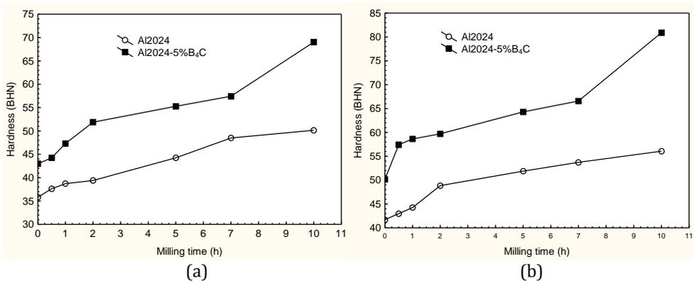
**Fig. 5** The change of hardness of Al2024 alloy and Al2024- 5%B<sub>4</sub>C composite, (a) 300 MPa, (b) 400 MPa
