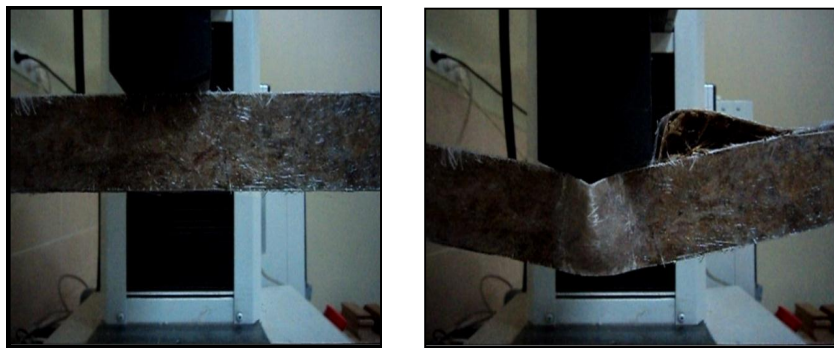
Fig. 5 Beginning of bending test and the moment of application of the force of F max when testing banana / glass fiber bio-composite
