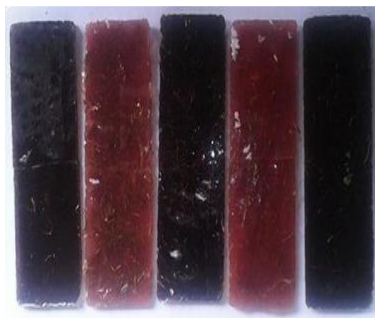
Fig. 3 Representative produced polyester hybrid composites
