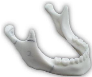
Fig. 7 Rapid prototyping (RP) model of human mandible
