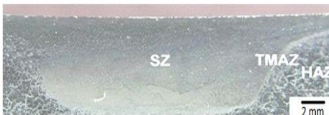
**Fig. 2** Macrostructure of Different Regions of FSW joints
