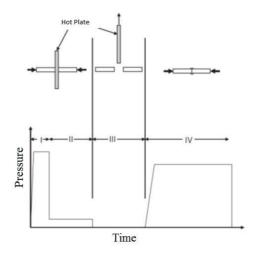
Fig. 6 Schematic pressure-time diagram showing four steps of HPW process [11]
