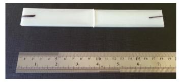
Fig. 5 Welding specimen joined by HPW
