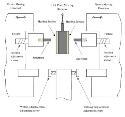
Fig. 4 Schematic diagram of HPW machine
