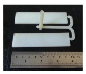
Fig. 2 Welding specimens produced by plastic injection molding
