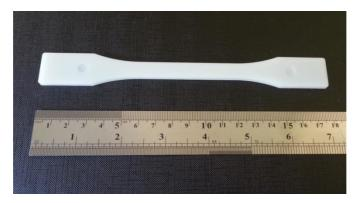
**Fig. 1** Tensile test specimen
