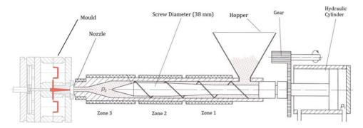
Fig. 3 Plastic injection molding machine
