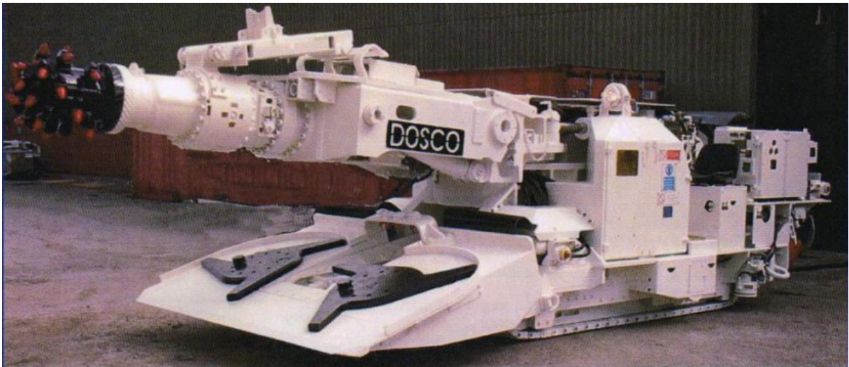
Figure 1. DOSCO MD1100 roadheader fitted with axial boom used in Tabas Coal Mine project (Dosco Ltd, 2008).
