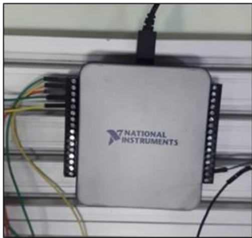
Figure 4. USB 6003 DAQ Card
