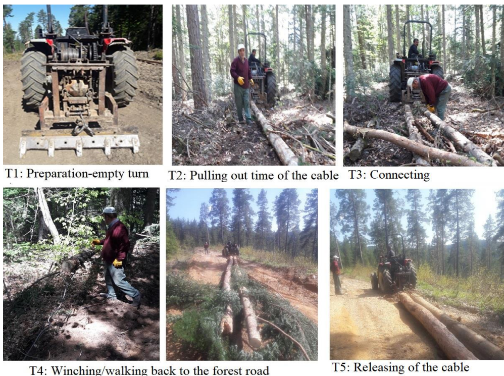
Figure 3. Work elements in a cycle during the winching at the harvesting site
