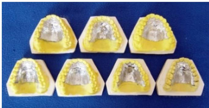
**Figure 1.** Ni-Cr and Co-Cr palatal plate samples.
