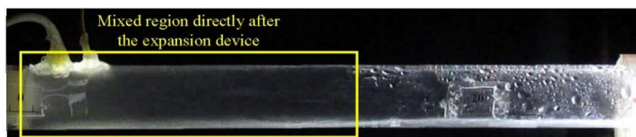
Figure 8. Homogenous flow (mixed flow) region of two-phase flow directly after the expansion device (flow direction from left to right)
