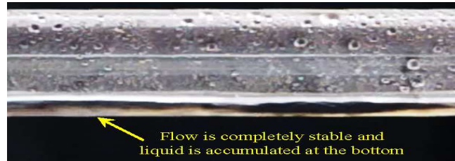
Figure 9. Stratified flow at 1600 mm from the inlet, \dot{m} = 10.2 g/s and x = 5.4\% (flow direction from left to right)
