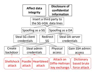
Fig. 3. Attack tree for MITM attack between SGs and the DA
