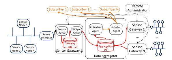
Fig. 1. General DA-PS platform architecture
