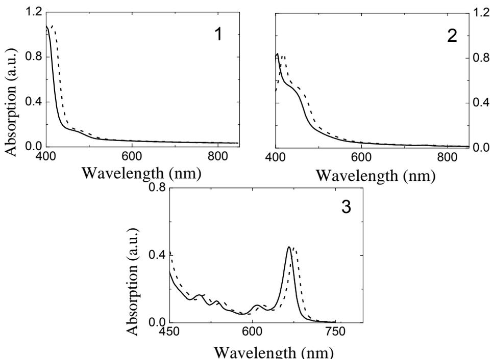
**Fig. 2.** Light absorption spectra of dye solutions (solid lines) and dyes adsorbed on TiO<sub>2</sub> (dashed lines) for (1) Biota orientalis, (2) Piper nigrum and (3) Glycyrrhiza glabra.
