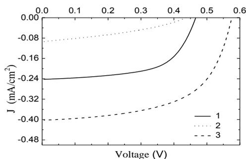
**Fig. 4.** Current density–voltage curves for the DSSCs sensitized by (1) *Biota orientalis*, (2) *Piper nigrum* and (3) *Glycyrrhiza glabra*, after grinding.
