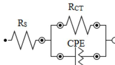
**Fig. 5.** The equivalent circuit for the DSSCs sensitized by natural dyes extracted with ethyl alcohol as solvent.
