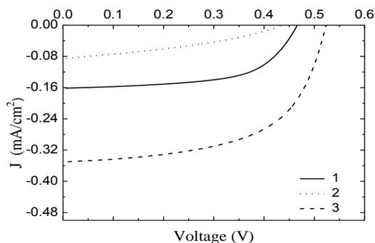
**Fig. 3.** Current density–voltage curves for the DSSCs sensitized by (1) Biota orientalis, (2) Piper nigrum and (3) Glycyrrhiza glabra, before grinding.
