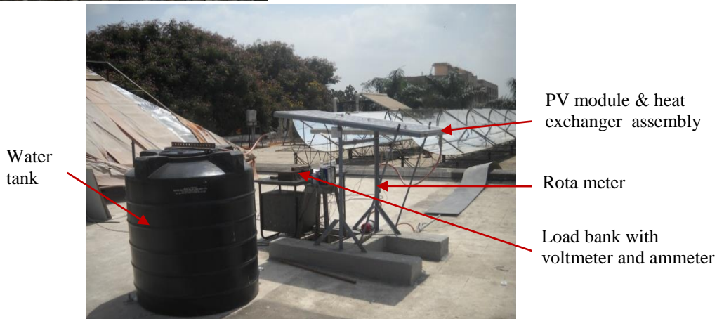
Fig. 3. Hybrid PV/T solar water system with measuring instruments
