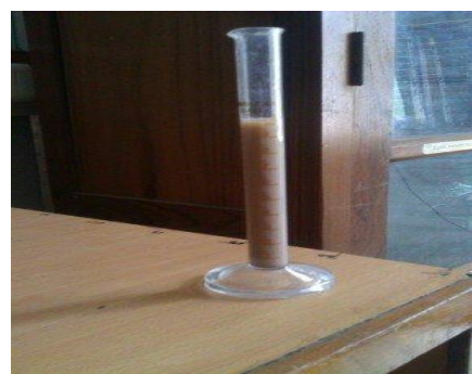
Fig. 7. Sedimentation of C- \text{TiO}_2 nanofluid
