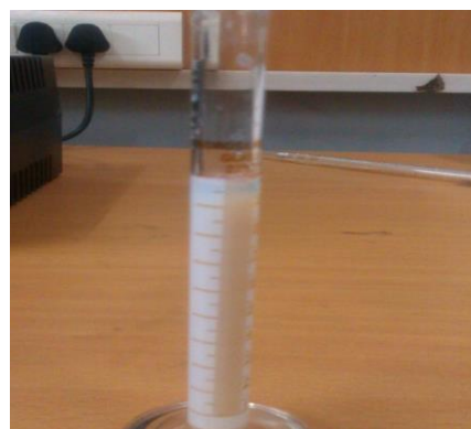
Fig 6. Sedimentation of \text{TiO}_2 nanofluid
